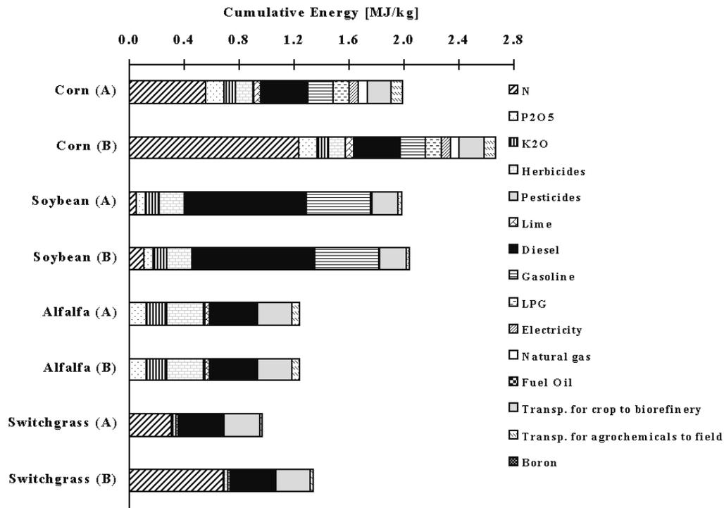
**Figure 3** Cumulative energy by input for producing biomass in 2000 disaggregated by input or process. "A" indicates carbon dioxide is a by-product of ammonia manufacture, and "B" indicates carbon dioxide is a waste in the ammonia production process. See text for details. LPG = liquefied petroleum gas.
