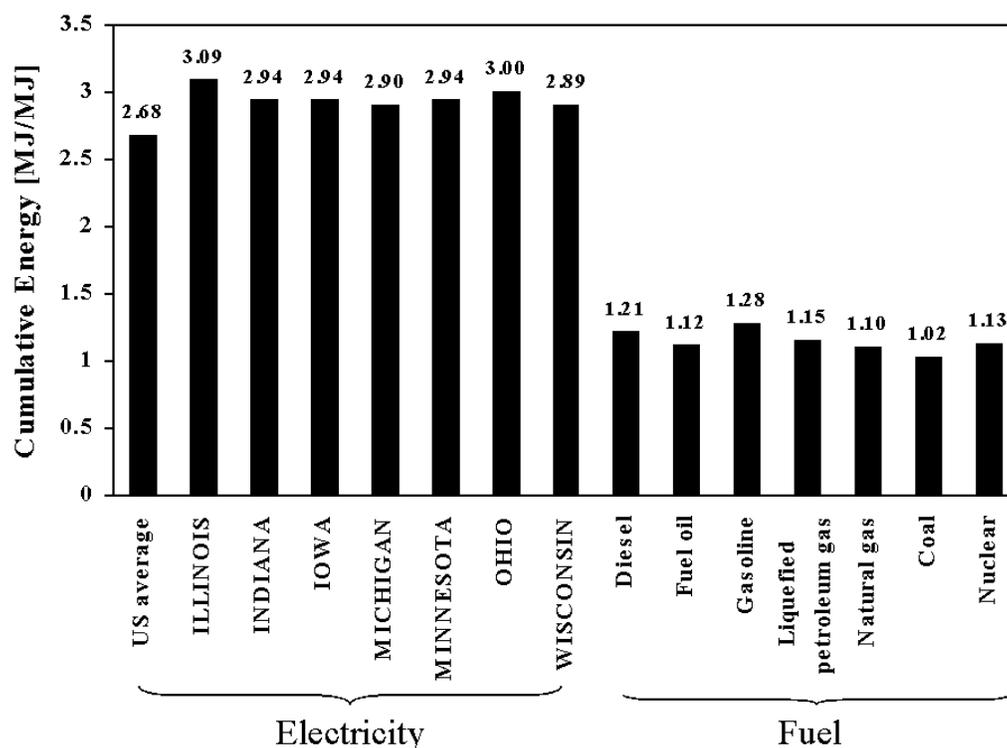
**Figure 2** Cumulative energy for electricity and fuel in 2000 (based on HHV).
