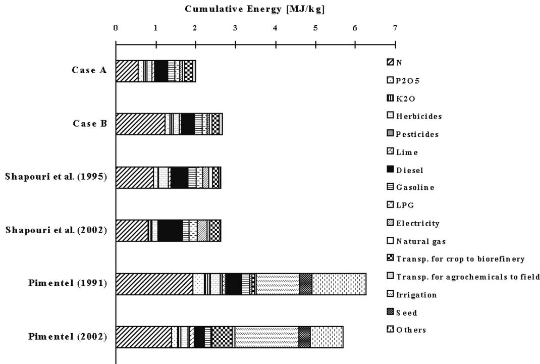
**Figure 6** Comparison of the cumulative energy requirement for corn production disaggregated by input or process. (Note: Pimentel's energy values are based on the LHV. Others include the energy requirement for manufacturing machinery, labor, and drying.)
