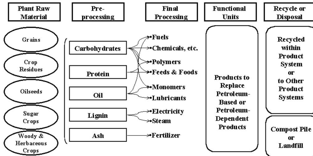
**Figure 1** Overall system definition for production and use of biobased products.
